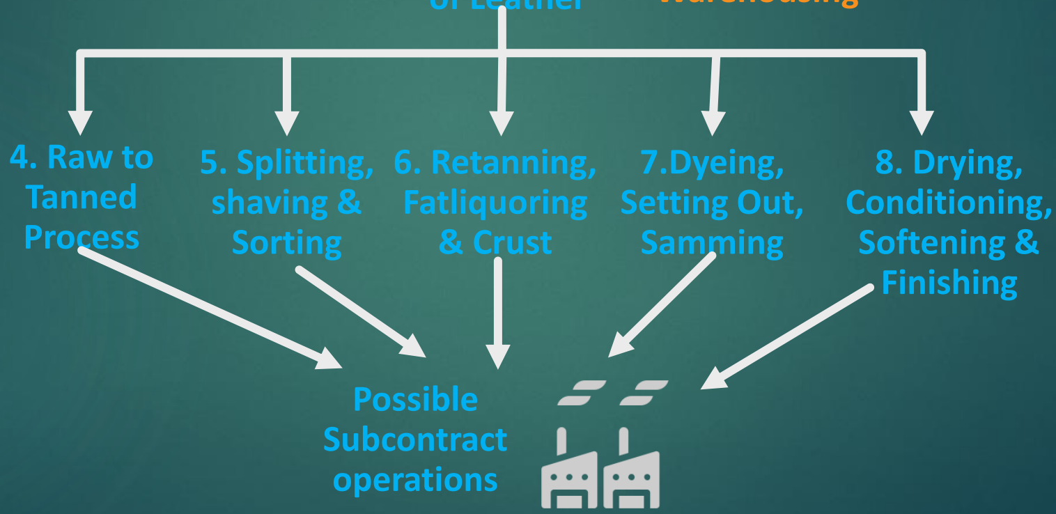
Flowchart of Key Processes in Leather Manufacture
