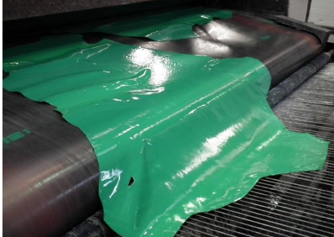
Grain patterning using special rollers.
