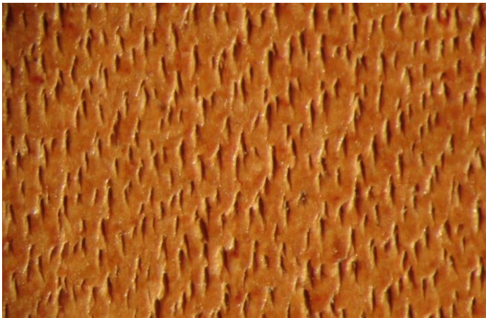
Grain surface of bovine leather (x20 mag).
